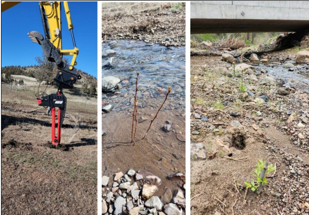
Left Photo – Expandable Tree Planter planting a cottonwood along Beaver Creek (Feb 15, 2024) Center Photo – Dogwood planted with Expandable Tree Planter (Beaver Creek) (March 28, 2024) Right Photo – Willow cuttings planted by hand along Dutchman Creek (May 21, 2024)
